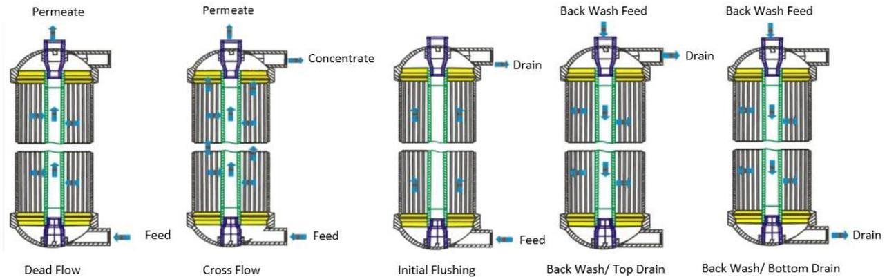
**5.2.1 Initial flushing:** The permeate valve is shut off, and an increased feed water stream is flushing the inner spaces of the membrane capillaries. This increased feed flow takes other contaminants that cannot be washed off just by water flush. This initial flushing usually takes 15-30seconds.
