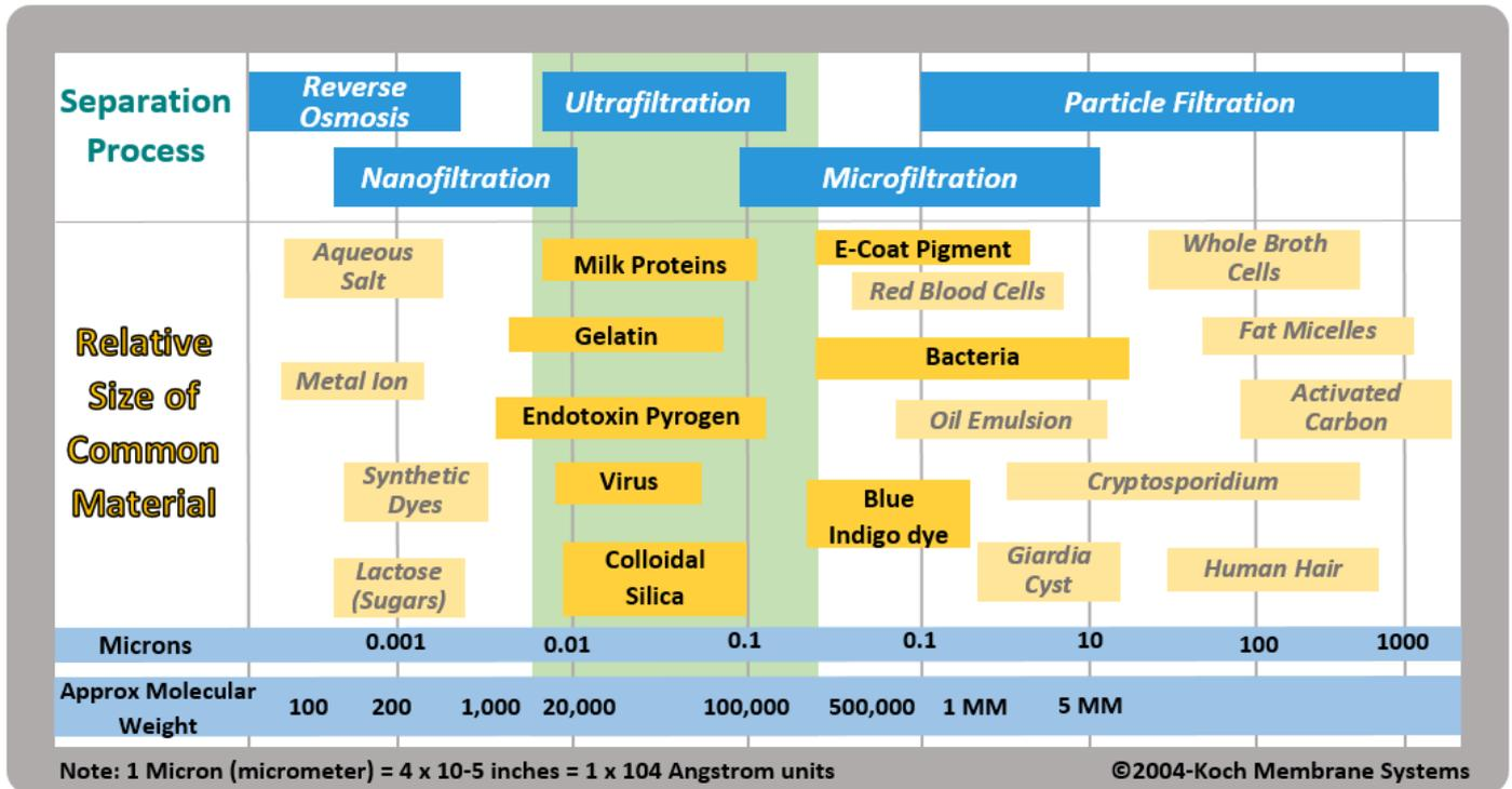
Retains oils, particulate matter, bacteria and suspended solids large macromolecules and proteins
