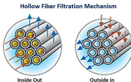
The second is **outside-inside** mode, in which the permeate passes through the fiber wall from shell side to the bore side under pressure.
